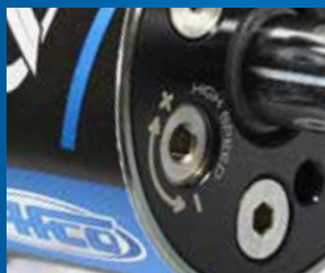
HIGH SPEED REBOUND ADJUSTMENT.
