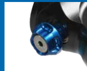
LOW SPEED REBOUND ADJUSTMENT.
