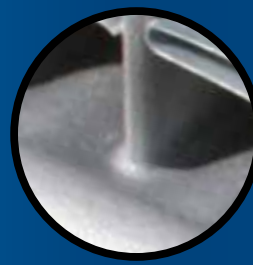
Clad Fillets on Both Sides
