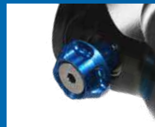
LOW SPEED REBOUND ADJUSTMENT.
