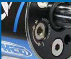
HIGH SPEED REBOUND ADJUSTMENT.
