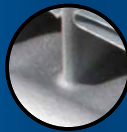
Clad Fillets on Both Sides
