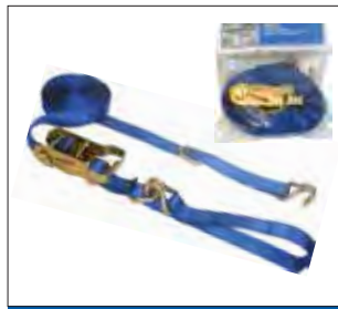
43887-10 Mini Ratchet Strap with D-Ring and Wire Hooks WLL: 1,000 lbs./454 kg. 1" x 16' Weight: 1.56 lbs./.71 kg. 43887-11 1" x 20' Weight: 1.69 lbs./.77 kg.
