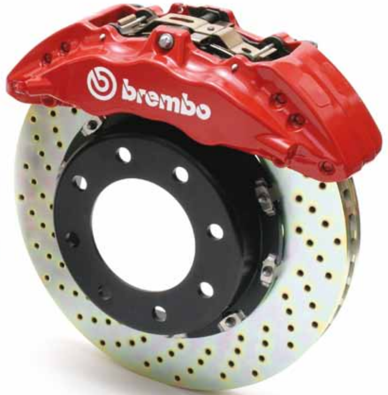
Two-piece "floating" rotor assembly
