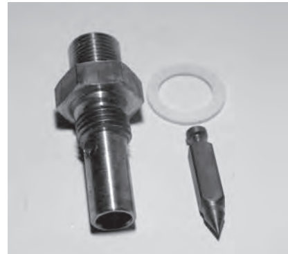
Carburetor Float Valve and Seat Reproduction of OEM 27382-33 float valve and seat, OEM 27402-33 gasket used on 1933-1965 Linkert carburetors. Stock No. 2880-3
