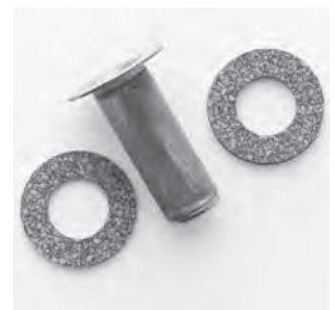
Gas Strainer Screen Quality duplicate of original brass screen assembly and gaskets. Fits Big Twins and 45's 1932-1965 OEM P/N 62265-32 screen, 62270-32 gasket. Stock No. 8927-3
