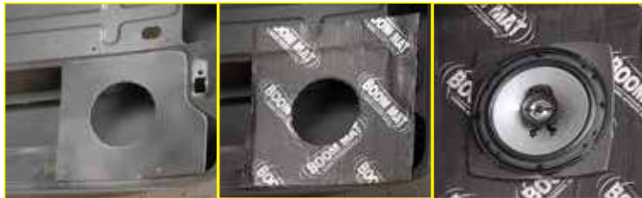
Remove speaker, apply material, re-install speaker
