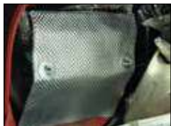
Protects electrical connections from engine and exhaust heat
