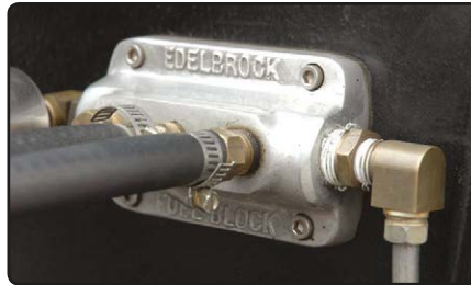
Fuel Block #1285 installed
