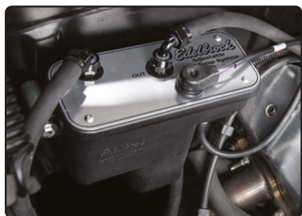
Universal EFI Sump Fuel Kit Installed
