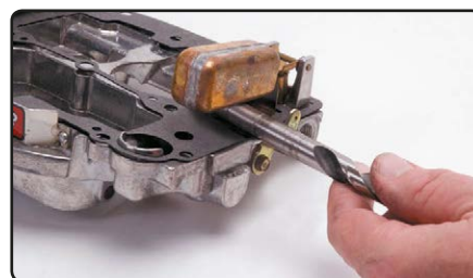
Checking float level with a 7/16" drill bit
