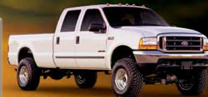
2003 FORD SUPER DUTY • 5.5" PERFORMANCE SYSTEM • 315/75R16 TIRES • 16X10 WHEELS W/ 4 5/8" BACK SPACING
