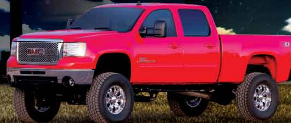
2008 GM C2500 • 8" PERFORMANCE SYSTEM • 37/14.00R18 TIRES • 18X9 WHEELS W/ 5" BACK SPACING
