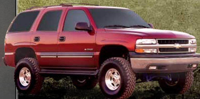
2003 GM C1500 Tahoe •6" PERFORMANCE SYSTEM •305/70R16 TIRES •16X8 WHEELS W/ 4 5/8" BACK SPACING
