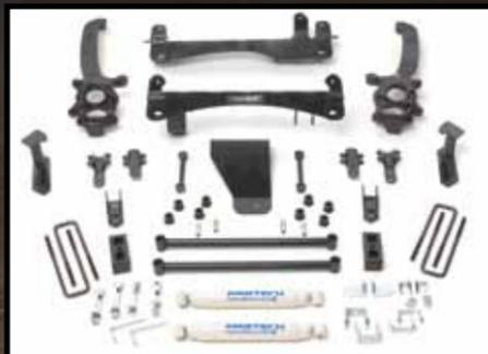
Lift is accomplished via a steel coilover shock spacer system retaining the stock ride characteristics of the vehicle. The Rack and Pinion remains in the factory location increasing installation time. Also included in this system is a 1/4" thick differential skid plate and Impact struts. Rear lift is accomplished with a Block and U bolt system.
