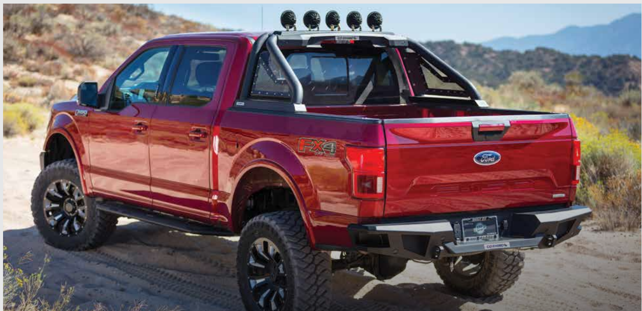
Power-actuated light mount bar kit
