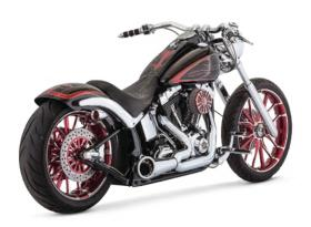
• Triple stepped headers 1.75" to 1.875" to 2.00" for increases of 15-18 HP and 13-15 foot lbs. of torque
