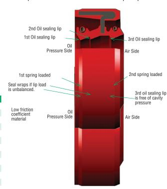
Functions smoothly during repetitive jumping. Seal life is 540,000 strokes, equal to 100 hours of continuous 28.8' jumps. Seal life exceeds current seals by 496,800 strokes (8 hours of continuous 28.8 foot jumps).
