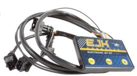
The GEN 3 is a piggy-back EFI controller because it does not replace the stock ECU, but rather monitors the signals to the injectors and makes fuel adjustments based on the mode settings. The GEN 3 has a push button interface allowing access up to 6 different modes to allow for quick fine tuning by the end user without needing a computer. The GEN 3 also is nitrous oxide compatible, and allows the user to add fuel thru the stock fuel injection when using nitrous oxide.
