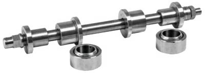
Specially-designed to upgrade the quality and feel of the driveline on your FXR or Touring model bike. These 7-piece kits convert the old-style Original Equipment parts to high-tech spherical bearings with CNC-machined precision spacers and collars.
