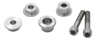
Solid riser bushing conversions eliminate flex in your handlebars often related to worn out rubber bushings. Made from stainless steel, 1/2"-13 x 1-3/4" riser bolts included. Will not fit Softail Deuce or Springer models.
