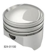
KB Hypereutectic alloy pistons are cast with a 16% high silicon content that has very high thermal barrier properties along with a low thermal expansion rate, allowing tight piston to cylinder wall clearances. This makes them ideal for air-cooled engines, offering optimal ring seal, quieter engine running and reduced wear. Hypereutectics are best suited for stock or mild compression ratios up to 10.5:1 running on pump fuel.
