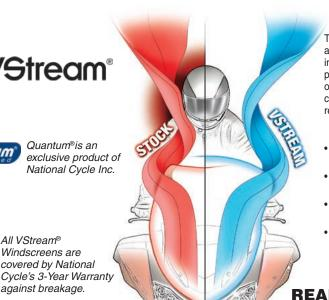
The VStream® gets its name from the unique shape and dimensional contours designed and engineered into the windscreen. The patented "V" profile helps push the turbulent wind out and away from the side of the rider's head, producing a quieter and more comfortable riding experience. This improvement also reduces wind noise and buffeting for the passenger.
