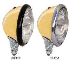
5-3/4" Solid brass headlights, deep drawn and formed from solid brass sheet, not cheaply plated like others... so they can be polished as often as you like, or allowed to age and acquire a nice patina. They have high beam indicator light, a 12-volt sealed beam, and include a bottom stud mount.
