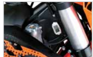
TTO shown mounted on the neck behind the forks on a 2008 KTM. This is a preferred mounting location for many installations. Mounted using the included 3M VHB tape, no drilling was required.
