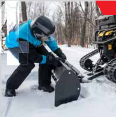
USE THE HANDLE TO CLICK THE FRAME IN PLACE
