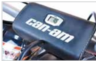
TTO shown custom mounted in bar pad. Use a knife to carefully carve out the recess for TTO to fit in. Use spray adhesive to hold the pad cover down tightly. This is a custom application, bar pads not available from Trail Tech.
