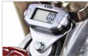
TTO shown mounted with universal mount at top of gas tank to Honda CRF450R 2009.
