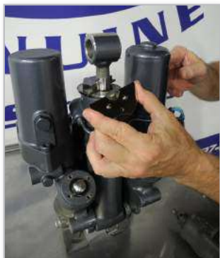
1. Place Two Piece Adapter On The Cap
