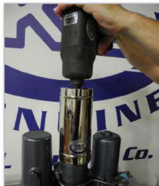
2. Place Impact Wrench Into Socket & Remove Cap
