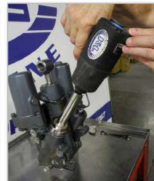
2. Attach Impact Gun Into The Socket & Remove The Cap
