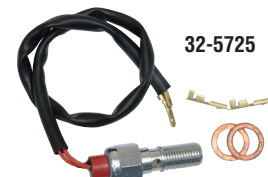
SINGLE BRAKE LIGHT BANJO BOLT 32-5725 Single, 3/8"-24 for 10mm 32-5726 Single, 7/16"-24 for 12mm
