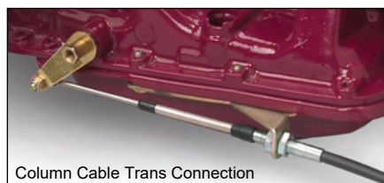
Column Cable Trans Connection
