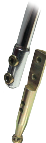
S10 Manual Shift Lever Adapter Installed in Factory Shifter.
