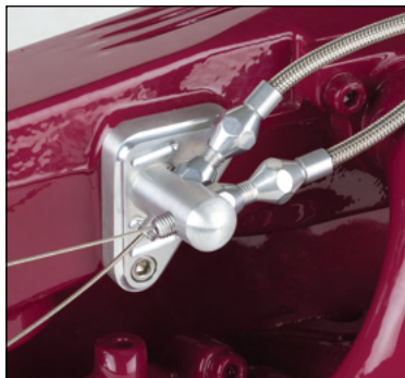
'88 and earlier throttle body end fitting shown
