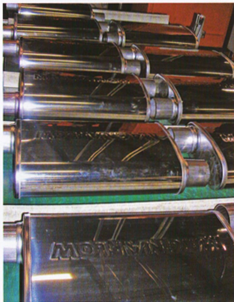
MagnaFlow performance mufflers are now produced by precise robotic welding equipment.
