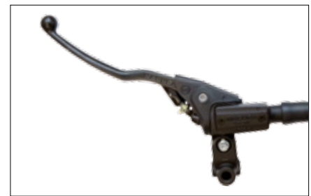
167 AXIAL MASTER Ø 9,5 Street (Light operation) ORDER CODE 0723295 Max. slave stroke: 8-10 mm* Ø 10,5 Street (Sports clutch) ORDER CODE 2700185 Max. slave stroke: 10-12 mm* Full details on page 27 167 Street Master – switch, mirror clamp and black street lever included
