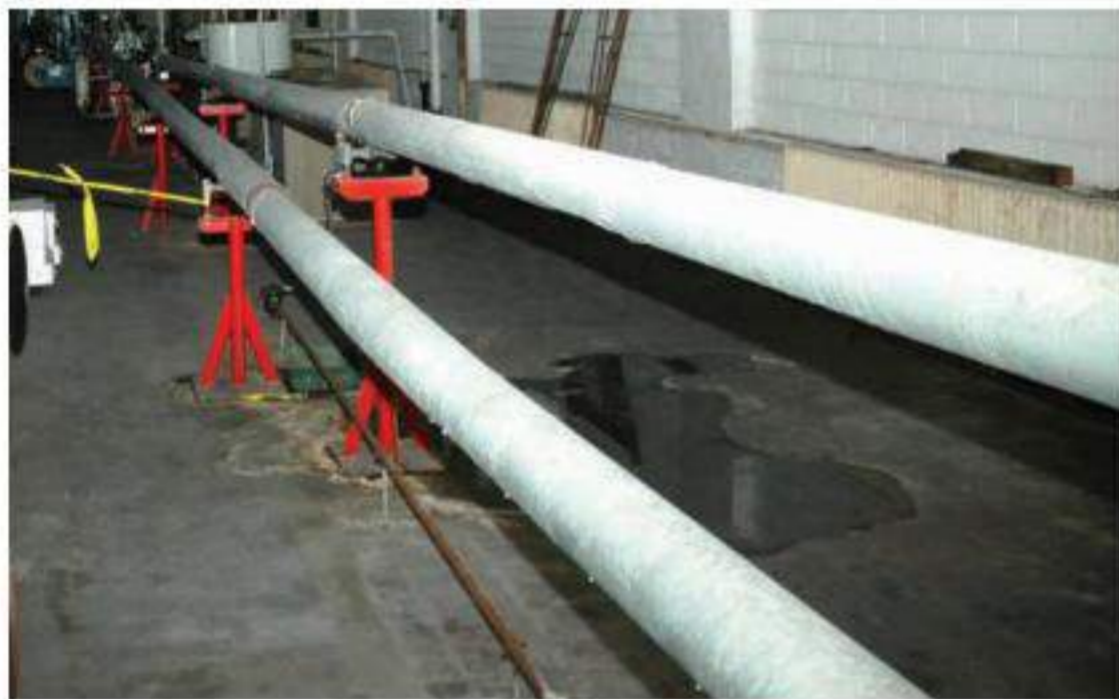
The wire travels 250 feet through these long tubes on the right in order to cure and cool the wire after manufacturing.
