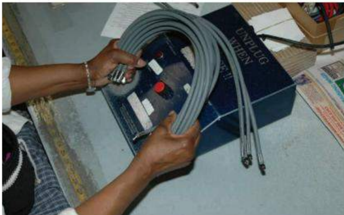
Before a plug boot is installed, each wire undergoes testing to ensure the quality of the crimp and the wire's conductivity. The plug boot is then installed, the wire is packaged and is ready for delivery.
