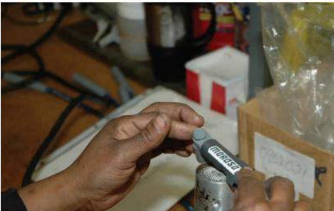
Moroso Ultra 40 Race Wire Sets receive a fiberglass reinforced silicone outer sleeve which requires a heat shrink sleeve at the boot in order to seal off the whole assembly.
