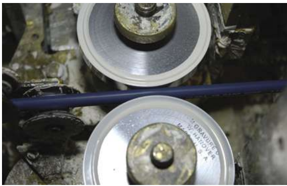
These print wheels are laser engraved with the Moroso and Ultra 40 Race Wire logos. At the end of the forming line, the wheels pick up ink and print on both sides of the wire.
