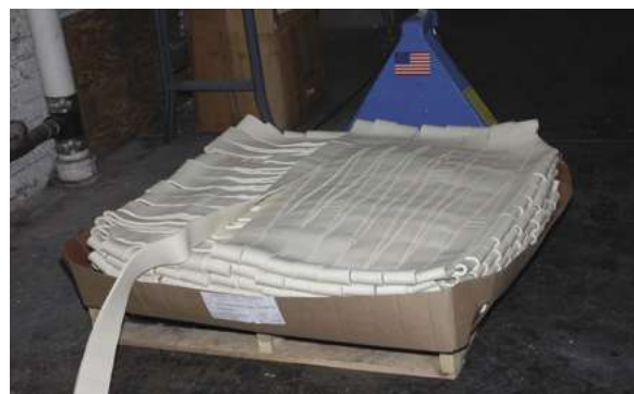
The rubber cover material for the center conductor starts out in this ribbon-like form. It's fed into a tube that heats and feeds it through a series of collets to form it around the center conductor.
