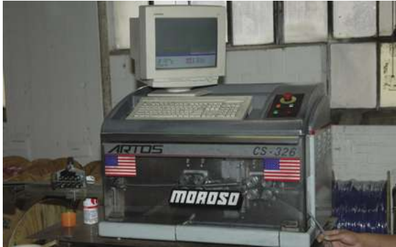
This automatic machine cuts the wire from the bulk spools to specified lengths and strips back the insulation on both ends prior to the terminal end crimping process.
