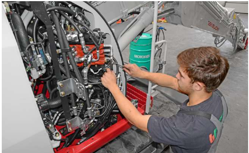
Under pressure: The valve set on this Takeuchi compact excavator controls all hydraulic functions.
