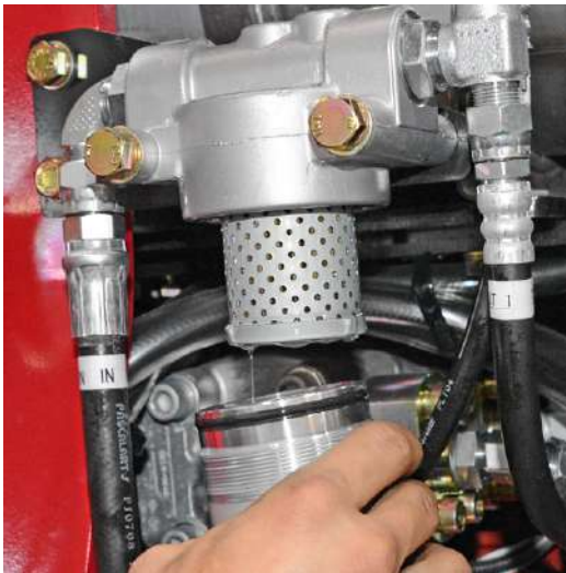
Clean: Corex HVLP-D ZF holds dirt particles in suspension and carries them to the filters.
