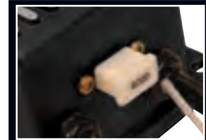
The 6 HVC-L Ignition features a built-in rev limiter.
