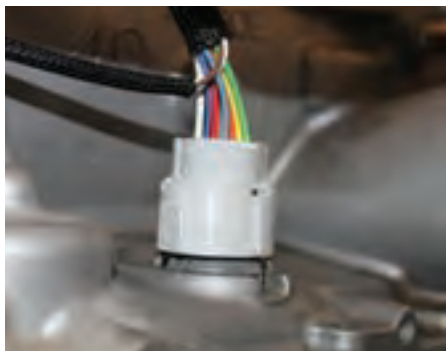
The Atomic Transmission Controller is easy to connect with OEM style connectors.
