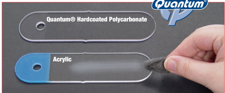
We use a steel wool scratch test to demonstrate the abrasion resistance of Quantum hardcoated polycarbonate (top) against acrylic (bottom).
