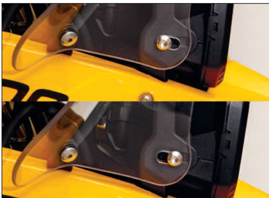
These VStream Windscreens use the headlight as an additional mounting point while maintaining complete headlight adjustability.
