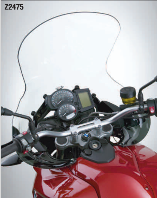
The structural side deflectors not only support a taller, touring-sized windscreen, they also help reduce updrafts.
