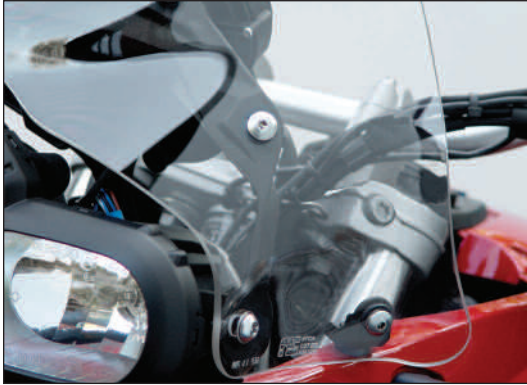
The lower contours add strength and rigidity.
