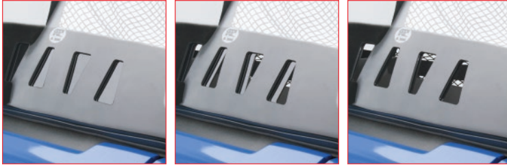
National Cycle's 3D-formed N30002 windshield for the Honda® Pioneer features an easily adjustable air vent.
