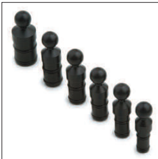
Z6405 BMW Steering Stem Mount Universal stem mount fits the steering stem nut of the 2010-14 S1000RR. Uses an O-ring shaft that gets progressively tighter as it is installed. Mounts devices center of the top triple clamp. Includes O-ring posts in 13mm, 16mm, 17mm, 18mm, 19mm and 24mm.
