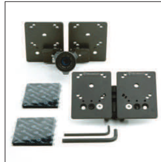
Dual Top Plate Z6458 Black Z6448 Silver Z6449 Chrome Mount two devices to the same mount! Dual 4-hole AMPS pattern 3.0" x 2.25" plates swivel independently.
