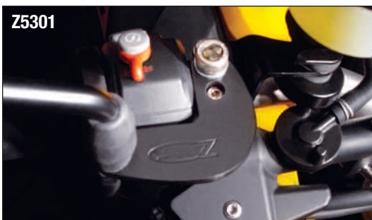
The Z5301 Mirror Deflectors include drilled access points for the OEM handlebar control adjusting screws.
