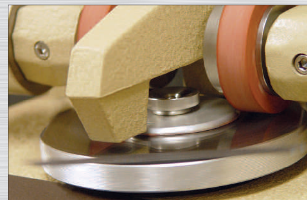
Scientific laboratory monitoring and measurement instruments test the surface wear on both hardcoated and uncoated windshield materials.
