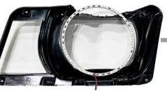
Place your ORACLE Halo ring in the diffuser location. Remove the 3M backing and make sure the wire is not in the way.
