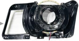
Re-install the Bezel and tighten down the four T-10 Torx Screws
