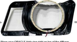
Place your ORACLE Halo ring right on top of the diffuser. Remove the 3M backing and make sure the wire is not in the way.
