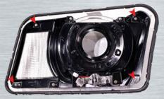
Remove these four T-10 Torx Screws first.
