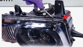
Use a flat head screwdriver to softly seperate the lens and the housing. Continue all the way around the headlight until it begins to part.
