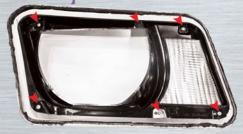
For the Non-RS models without projectors, you just have to remove these six T-10 Torx Screws.
