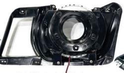
Re-install the Bezel and tighten down the four T-10 Torx Screws
