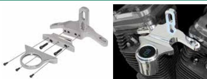
THIS GROUPING SHOWS A POLISHED YE-MM-04 MOTOR MOUNT WITH A CHROME YE-GA-01 GAUGE ADAPTOR AND A CHROME YE-T-17 GAUGE TOP. THE YE-GA-01, WHEN COMBINED WITH A YE GAUGE TOP, WILL LET YOU ATTACH A TACH OR SPEEDO TO YOUR MOTOR MOUNT, CLEANING UP YOUR HANDLEBARS.
