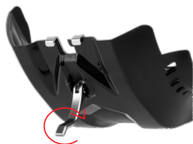
2 Use the quick install lever clamp to hold the skid plate on the bike.
