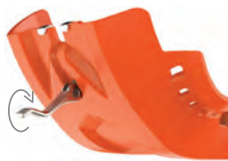
2 Use the quick install lever clamp to hold the skid plate on the bike.
