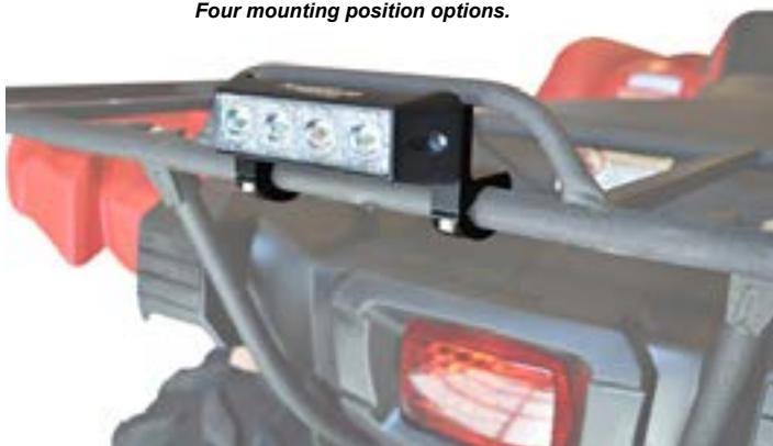
66005 - mount under or over your rear rack. Four mounting position options.
