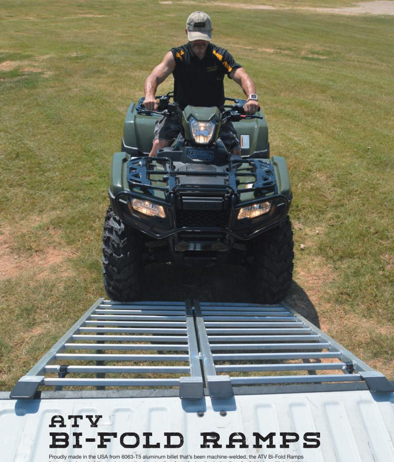
Proudly made in the USA from 6063-T5 aluminum billet that's been machine-welded, the ATV Bi-Fold Ramps feature vinyl-coated tips and a security strap to allow for safer loading/unloading. Available in multiple widths to accommodate almost any ATV.
