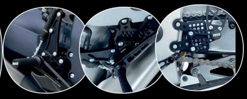
Maximise your potential, tune your machine to your exact requirements. R&G Racing Adjustable Rearsets are milled out of lightweight aluminium for
