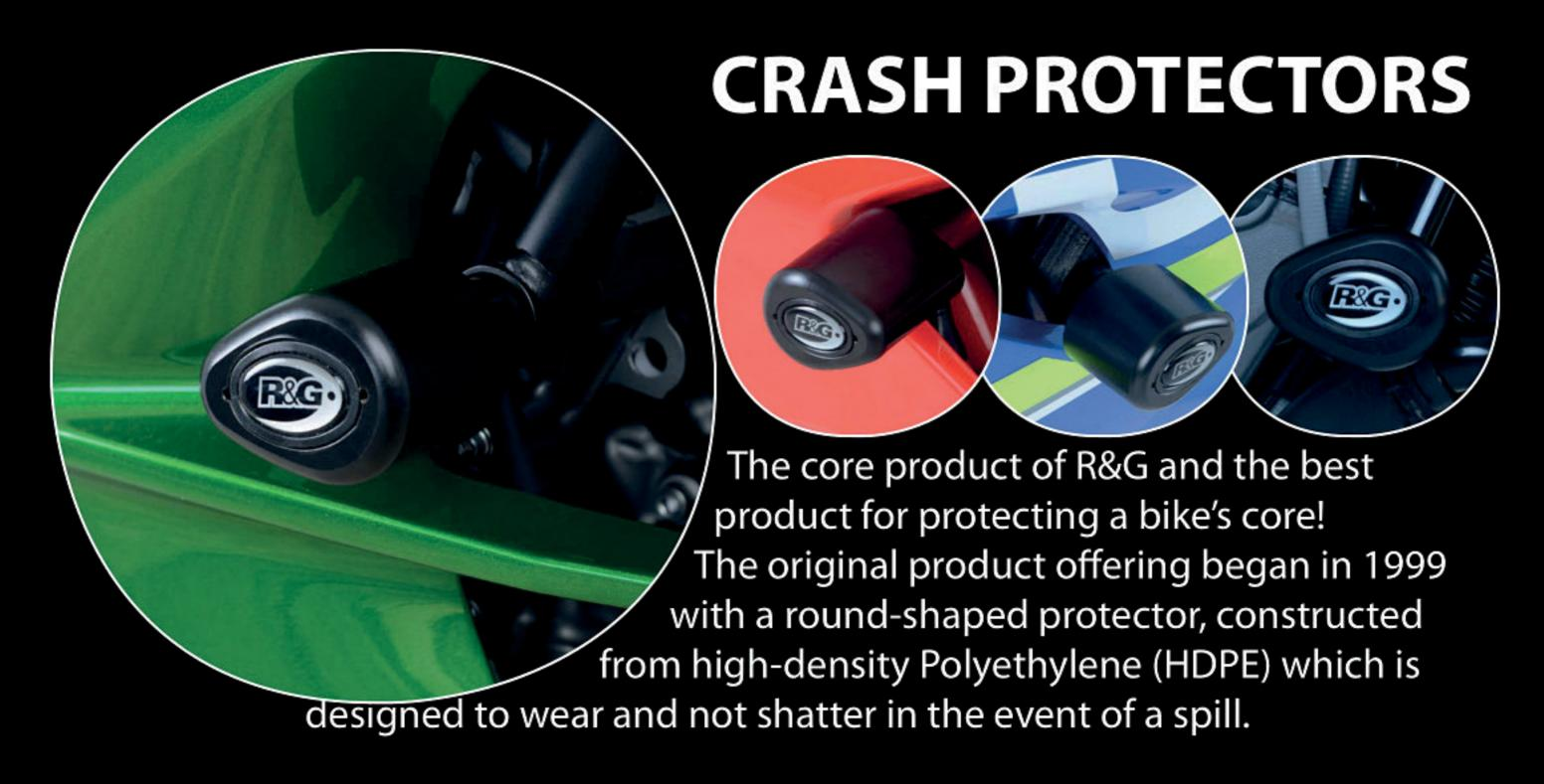
With the initial 'bung', R&G introduced two industry firsts; by adding a metal sleeve into the bung, it increased its strength and allowed the fitter to correctly torque the protector down. The second was to use a particular grade of steel bolt that helps absorb impacts by bending when it exceeds a certain load, rather than snapping or twisting its mounting point on the bike.
