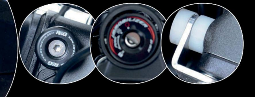
These Lockstop Savers have been specially designed for the extremes of a motorcycle crash, the lockstops on the yoke can easily be broken off, and this
