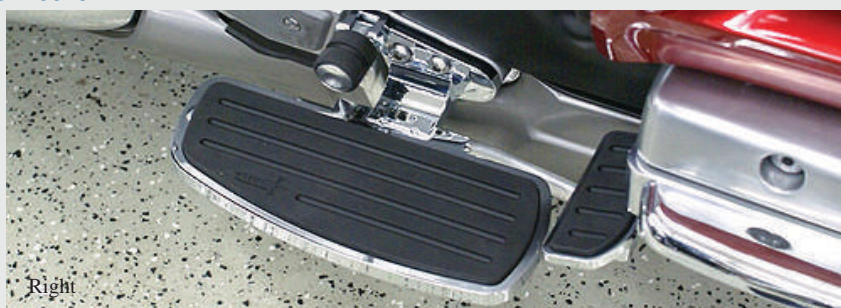
GL18020 Driver Boards fold up and include a kickstand extension
