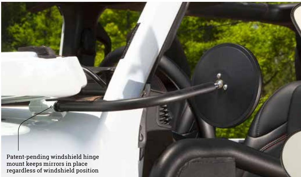
Patent-pending windshield hinge mount keeps mirrors in place regardless of windshield position
