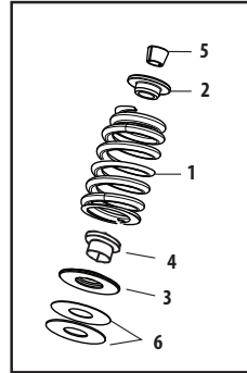
.650" Lift Sidewinder® Valve Springs
