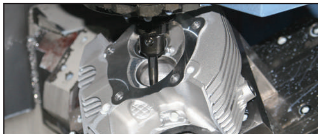
Digitized port shapes are faithfully reproduced in X-Wedge cylinder heads on our 5-Axis CNC machining center. Intake port, exhaust port and combustion chamber are all modified. This head will be assembled with new valves and high lift valve springs to complete the package.
