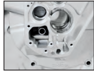
Relocated oil scavenge pick-up reduces oil carry-over by increasing oil scavenge efficiency.
