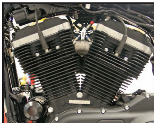
S&S cylinders match the fin profile on 1986–'03 cylinder heads. Although there is a slight difference in the fin profiles of S&S cylinders and stock 2004–'18 cylinder heads (shown above), the look is generally not considered to be objectionable. You decide!
