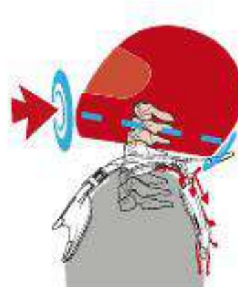
POSTERIOR HYPERTRANSLATION: extreme movement of head and helmet, rearward on the neck.
