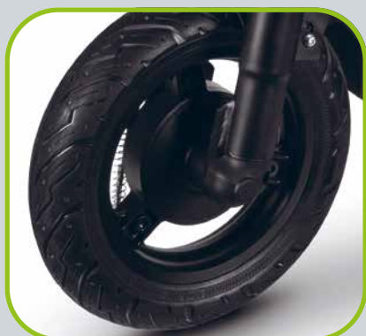
10 Inch honeycomb tubeless tyres.
