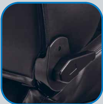
Tilt lever and back adjustment on both sides.
