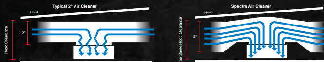
Drop base air cleaner assembly means increased filter area for increased airflow with the same low hood clearance.
