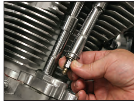
When a Quickee adjustable pushrod is collapsed, it can easily be installed or removed from an assembled engine.
