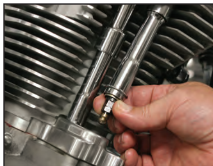
When a Quickee adjustable pushrod is collapsed, it can easily be installed or removed from an assembled engine.
