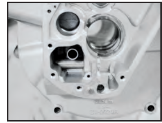
Relocated oil scavenger pick-up reduces oil carry-over by increasing oil scavenger efficiency.
