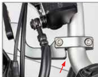
A stopper that reduces damage to the exterior due to a fall.
