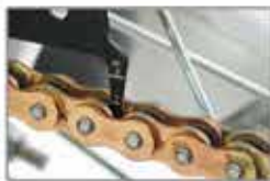
B. Lower the measuring nib. Extension rate will be shown on measuring nib where it touches the chain roller.
