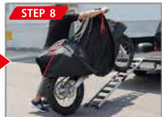
Wrap a tie-down soft hooks around the handlebar then load on a truck.
