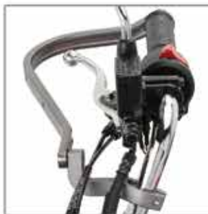
The specialized handle clamp shape avoids brake hose and wire interference and allows perferrad angle setting.
