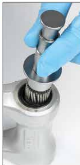
Insert the tool into the linkage carefully and gently so as not to slip the bearing needles. Push the shaft to extrude grease to attach the bearing needles inside the shell.
