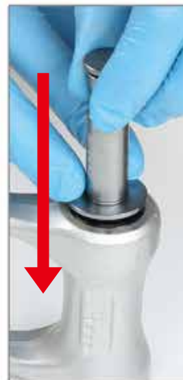
The bearing needles will be placed inside the shell by pushing the slide body further.
