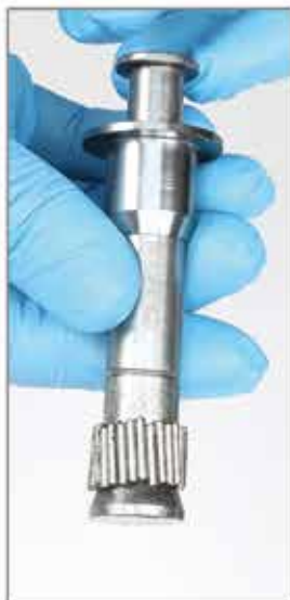
Attach the bearing needles on the slide body. *Can not place all bearing needles on the injection body.
