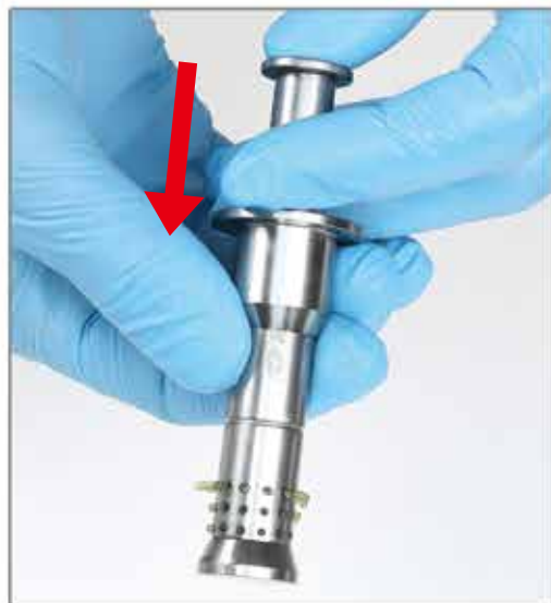
Push the shaft and extrude the grease to easily stick the bearing needles.
