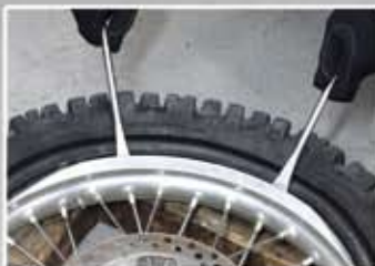
1. Insert the tire bead into the wheel rim after installing the tube.
