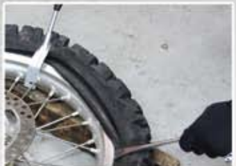
4. Tire bead won't come off with bead keeper. Smooth and easy operation.
