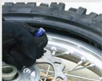
STEP4: Pull on the air valve wire. The air valve will appear.
