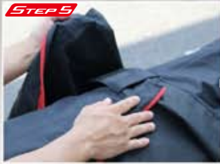
Lace the hook and loop fastener into the loop on the rear fender and secure.
