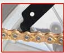
A. Lightly attach Chain Checker on the chain roller.
