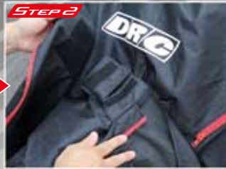
Lace the hook and loop fastener into the loop on the front fender and secure.
