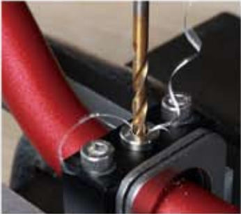
Comes with 5 mm hole drilling guide for handlebar.
