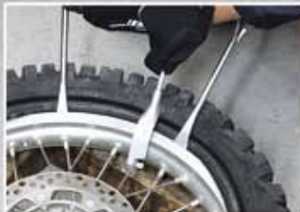
2. Insert lever part of the bead holder into the wheel rim and hook over spoke as shown above picture.
