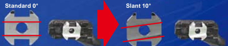
Turn over spacers to change hand guard angle.
