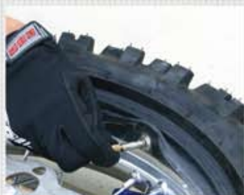
STEP2: Install valve puller head on air valve on the tube.
