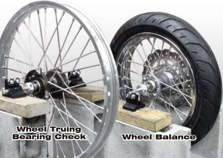
Lock wheel rod for wheel truing and bearing check.
