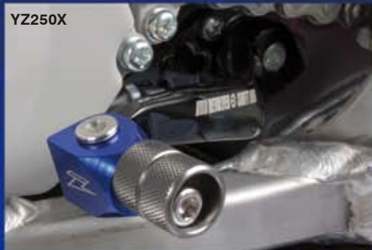
Shift tip is color anodized with ZETA laser print logo.
