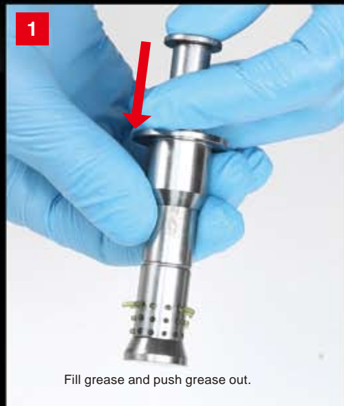
Place your bearing needles on injector body.
