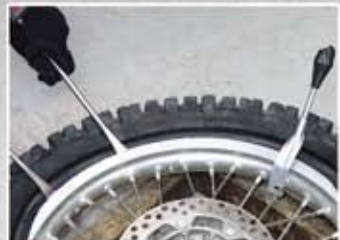
3. Keep the tool inserted and insert the tire bead into the wheel rim.
